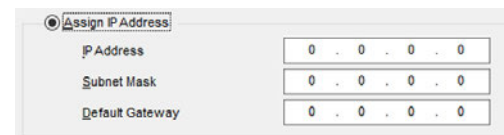
FIG. 22 – MANUALLY CONFIGURING THE IP ADDRESS OF THE MACHINE
