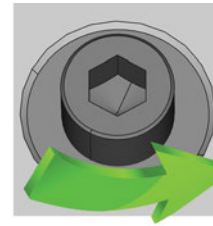
FIG. 44 – SCREWING DOWN THE SCREW TO IMMOBILIZE THE BLOCK
